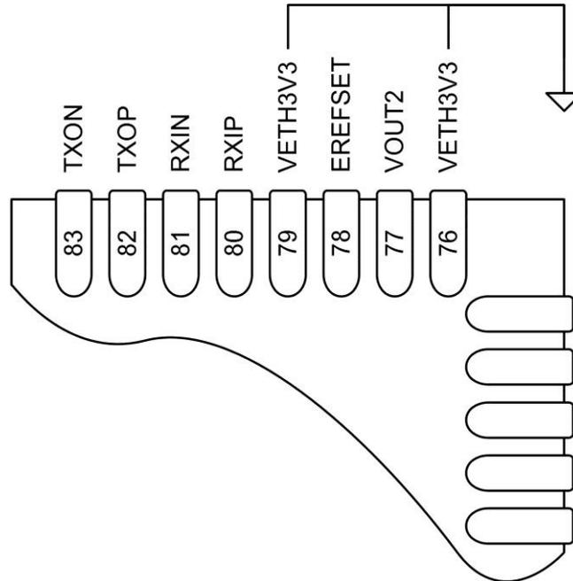
Figure 6-8 Unused Ethernet Connection (QFN)
