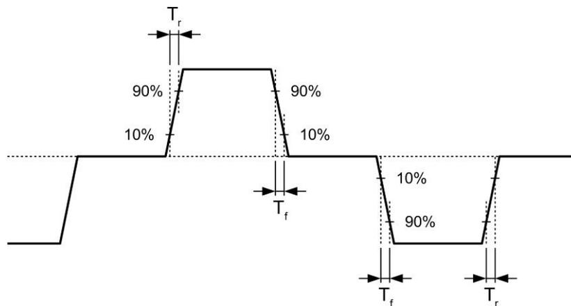
**Figure 5-2 100Base-TX  $T_{r/f}$  Timing**
