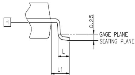
Figure 7-3 LQFP-100 Package Dimensions
