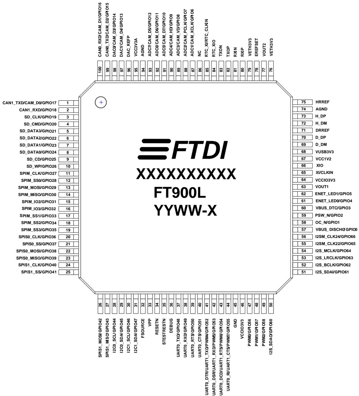
Figure 3-5 Pin Configuration FT900L (top-down view)
