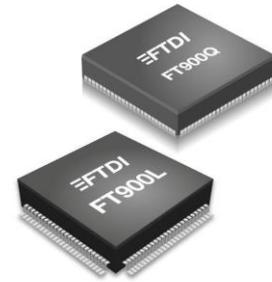
The FT90x series includes the FT900, FT901, FT902 and FT903 which are complete System-On-Chip 32-bit RISC microcontrollers for embedded applications featuring a high level of integration and low power consumption. It has the following features:
