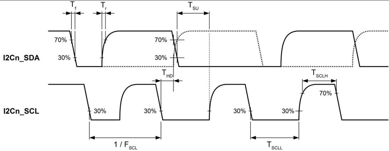
Figure 5-5 Definition of I<sup>2</sup>C Timing F/S mode
