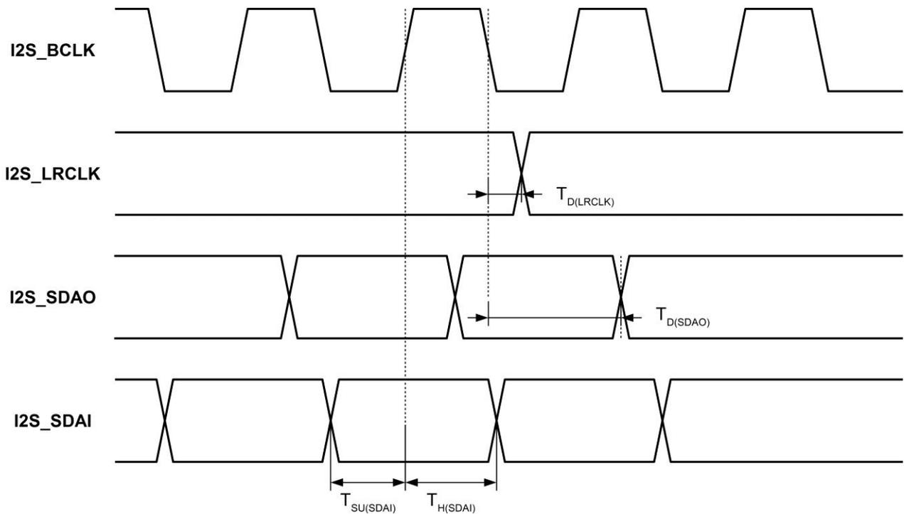
**Figure 5-9 Definition of I<sup>2</sup>S Master Timing**
