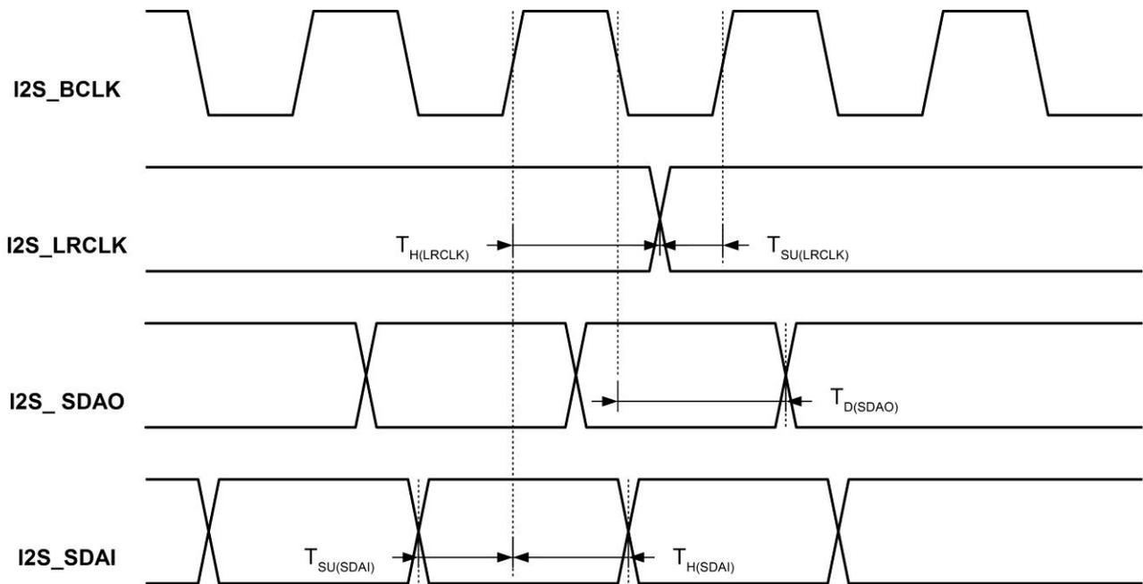
**Figure 5-10 Definition of I<sup>2</sup>S Slave Timing**
