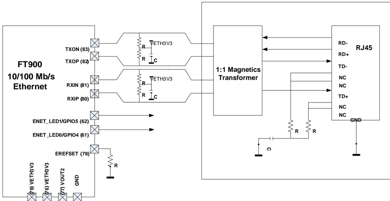
Figure 6-7 10/100Mbps Ethernet Interface
